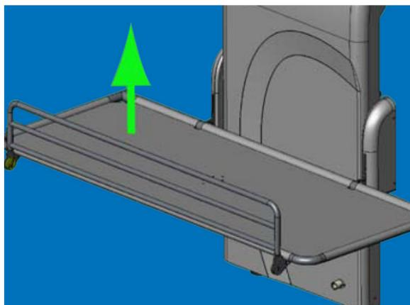
Operating the guard. Folding the guard. Lift the guard upwards.
