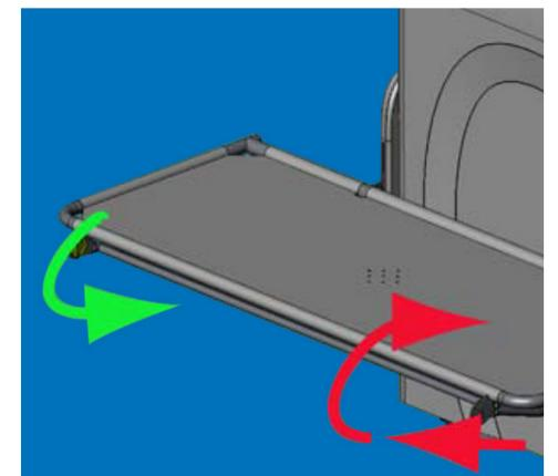
It will then lock under the bed. To replace the guard lift it slightly towards you, it will release, rotate upright and drop into position.
