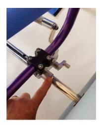
Once fully inserted and ensure security button is locked in place
